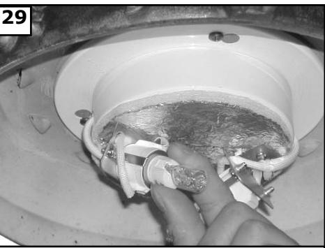
Install the 2 50 watt halogen bulbs. Do not touch bulb surface as oily residue from skin can cause the bulb to explode.
